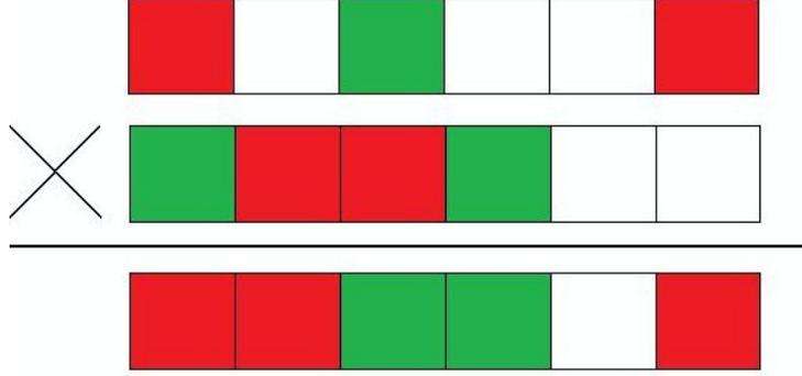
A graphical representation for multiplying  $G \sim (-, +, +, -, 0, 0)$  by  $F \sim (+, 0, -, 0, 0, +)$  to obtain  $FG \sim (+, +, -, -, 0, +)$
